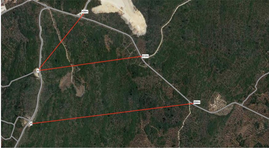
Fig. 2.10: Measurement location for the rural experiment. “A” and “B” represent gateway locations while the labels with the distances represent node locations. (Adapted from Google Maps.)
